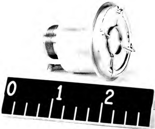
FIGURE 12-5.—The NRL X-ray photometer flown on Solrad 1. (U.S. Navy photograph.) Scale is in inches.
